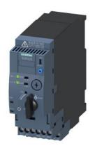
SIRIUS Compact load feeder DOL starter 690 V 110...240 V AC/DC 50...60 Hz 0.32...1.25 A IP20 Connection main circuit: plug-in, without terminals Connection auxiliary circuit: screw terminal
