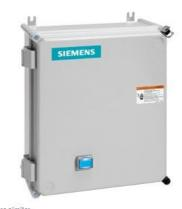
Non-reversing motor starter, Size 2 1/2, Three phase full voltage, Amb. compensate bimetal OLR, Contactor amp rating 60A, Non-combination type, Enclosure type 4X fiberglass, Water/dust tight noncorrosive
