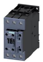
Power contactor, AC-3 65 A, 30 kW / 400 V 1 NO + 1 NC, 84-155 V AC / DC with varistor 3-pole, size S2 screw terminals
