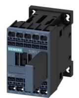
Power contactor, AC-3 7 A, 3 kW / 400 V 1 NO, 110 V AC, 50 Hz 120 V AC, 60 Hz, 3-pole, Size S00, Spring-type terminal RC element 3RT2916-1CC00 plugged on
