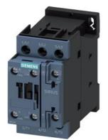
power contactor, AC-3 25 A, 11 kW / 400 V 1 NO + 1 NC, 200 V AC, 50 Hz, 200-220 V, 60 Hz, 3-pole, Size S0, screw terminal
