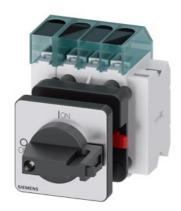
Load disconnector 3LD3, lu 25 A Main switch 3-pole + N Rated operating capacity at AC-23 A at 400V 9.0kW Front plate mounting Basic switch with Central hole mounting 22.5mm Toggle drive black 48x48 mm with auxiliary switch 1OE + 1S
