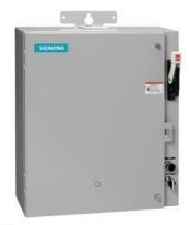
Pump control panel, Size 3 1/2, Three phase full voltage, Solid-state overload relay, OLR amp range 50-200A, 110V 50Hz / 120V 60Hz coil, Standard type contactor, 125A circuit breaker, HOA Sel Sw. <(>&<)> Start P.B., Enclosure NEMA type 3/3R, Weather proof outdoor use
