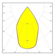
Dimensions: 110.0 mm x 110.0 mm Height: 57.30 mm ~60° wide beam compatible with BJB and B+W connectors
