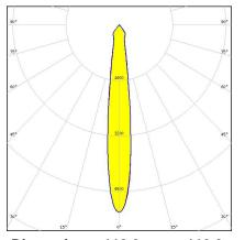
Dimensions: 110.0 mm x 110.0 mm Height: 57.30 mm ~10° spot beam. Clean appearance with no additional attachment interface.
