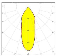
Dimensions: 110.0 mm x 110.0 mm Height: 57.30 mm ~35° medium beam
