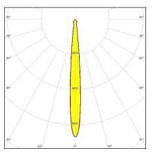
Dimensions: 110.0 mm x 110.0 mm Height: 57.30 mm ~10° spot beam compatible with BJB and B+W connectors
