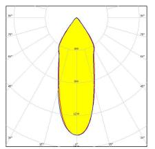
Dimensions: 110.0 mm x 110.0 mm Height: 57.30 mm ~35° medium beam. Clean appearance with no additional attachment interface
