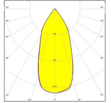
Dimensions: 110.0 mm x 110.0 mm Height: 57.30 mm ~50° medium beam
