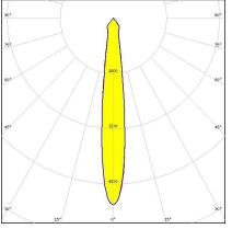
Dimensions: 110.0 mm x 110.0 mm Height: 57.30 mm ~10° spot beam
