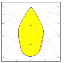
Dimensions: 110.0 mm x 110.0 mm Height: 57.30 mm ~60° wide beam. Clean appearance with no additional attachment interface.
