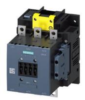
Power contactor, AC-3 185 A, 90 kW / 400 V Coil AC 50/60 Hz and DC 96-127 V x (0.8-1.1) F-PLC input 24 V DC 3-pole size S6 Auxiliary contacts 2 NO + 2 NC Main circuit: Busbar Control and auxiliary circuit: screw terminal
