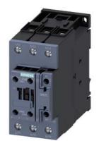
Power contactor, AC-3 80 A, 37 kW / 400 V 1 NO + 1 NC, 220 V AC 50/60 Hz, 3-pole Size S2, screw terminals
