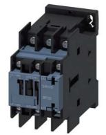
power contactor, AC-3 9 A, 4 kW / 400 V 1 NO + 1 NC, 110 V AC, 50 Hz 120 V, 60 Hz, 3-pole Size S0 ring cable lug connection
