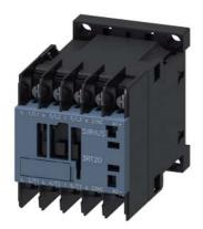
power contactor, AC-3 12 A, 5.5 kW / 400 V 1 NC, 24 V DC 3-pole, Size S00 ring cable lug connection
