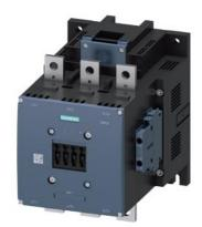
Contactor, AC-1, 690 A/690 V/40  $^\circ\text{C},$  S12, 3-pole, 240-277 V AC/DC, with varistor, 2 NO+2 NC, Connection rail/ screw terminal
