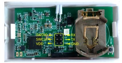
USB to TTL <- -> LDS01 RX <- -> TX TX <- -> RX GND <- -> GND
