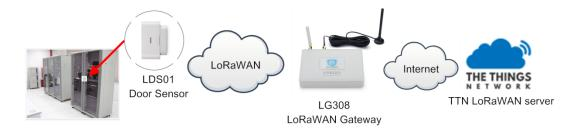
The LDS01 in installed on the door edge to detect the open / close event. And send the status to LoRaWAN server. The LDS01 will uplink two type of messages to the server.
