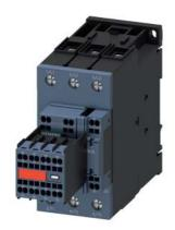
Power contactor, AC-3 80 A, 37 kW / 400 V with varistor; 2 NO + 2 NC 110 V AC, 50 Hz/120 V, 60 Hz 3-pole, size S2 Spring-type terminals Perm. mounted auxiliary switch
