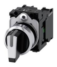
Selector switch, illuminable, 22 mm, round, metal, shiny, white, selector switch, short, 3 switch positions I>O<II, momentary contact type, actuating angle  $2x45^{\circ}$ , 10:30h/12h/13:30h, with holder, 1 NO, 1 NO, screw terminal, Z=20-unit packaging
