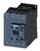
Power contactor, AC-3 50 A, 22 kW / 400 V 2 NO + 2 NC 20-33 V AC/DC varistor, 4-pole size S2 screw terminals 1 NO + 1 NC integrated
