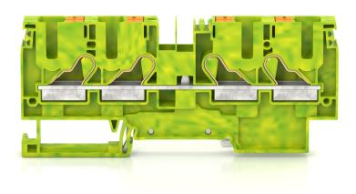
Protective earth terminal, Push-in connection, Mounting type: Mounting rail TS 35/7.5, Rated cross-section: 10 mm², Width: 10.1 mm, Colour: Green-yellow
