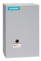
Mechanically held lighting contactor, Contactor amp rating 100A, 0 N.C. / 5 N.O. poles, 220VAC 50HZ/240VAC 60HZ coil, Non-combination type, Enclosure NEMA type 1, Indoor general purpose use
