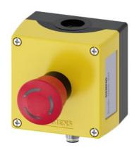
Enclosure for command devices, 22 mm, round, enclosure material plastic, enclosure top part yellow, 1 control point plastic, A=EMERGENCY STOP mushroom pushbutton red, 40 mm, rotate-to-unlatch, illuminated, 2x 1 NC, LED white 24 V, spring-type terminal, floor mounting, M12 connector (8-pole) bottom, insulated reserve conductors Pin assignment: PIN1=11, PIN2=12, PIN3=21, PIN4=22, Pin5=n.c., Pin6=n.c., Pin7=ground LED, PIN8=LED, one connection at 1 input F-DI, one connection at 1 output F-DO
