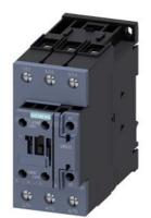
power contactor, AC-3 51 A, 22 kW / 400 V 1 NO + 1 NC, 110 V AC, 50 Hz, 3-pole, size S2, screw terminal
