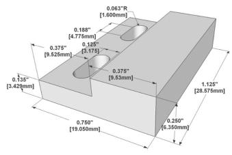
All measurements are in inches [millimeters]
