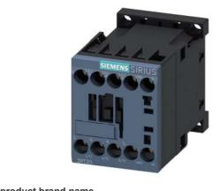
Power contactor, AC-3 12 A, 5.5 kW / 400 V 1 NO, 110 V AC, 50 / 60 Hz 3-pole, Size S00 screw terminal
