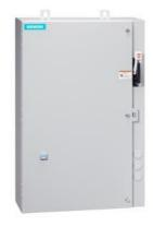
Non-reversing motor starter, Size 2 1/2, Three phase full voltage, Solid-state overload relay, OLR amp range 25-100A, 240V 50Hz / 277V 60Hz coil, Combination type, 100A non-fusible disconnect, Enclosure NEMA type 4/12, Water/dust tight for outdoors, Extra-wide enclosure
