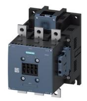
power contactor, AC-3 225 A, 110 kW / 400 V AC (50-60 Hz) / DC operation 21-27.3 V AC/DC auxiliary contacts 2 NO + 2 NC 3-pole, frame size S10 busbar connections drive: electronic with PLC interface 24 V DC screw terminal
