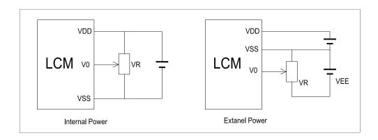
V<sub>DD∼</sub>V₀: LCD Driving voltage
