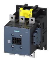
Power contactor, AC-3 265 A, 132 kW / 400 V Coil AC 50/60 Hz and DC 96-127 V x (0.8-1.1) F-PLC input 24 V DC 3-pole size S10 Auxiliary contacts 2 NO + 2 NC Main circuit: Busbar Control and auxiliary circuit: screw terminal
