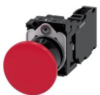
Mushroom pushbutton, 22 mm, round, plastic, red, 40mm, latching, pull-tounlatch mechanism, with holder, 1 NO+1 NC, screw terminal, with laser labeling, lower case
