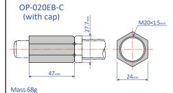
Note: When attaching, make sure that the side without a bearing chamfer is the impact surface.
