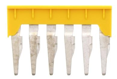
Insulated cross-connector, No. of poles: 6, Mounting type: Plug in, Width: 48.1 mm, Rated cross-section: 6 mm², Colour: Yellow
