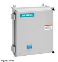
Non-reversing motor starter, Size 1, Single phase full voltage, Solid-state overload relay, OLR amp range 3-12A, Non-combination type, Enclosure type 4X fiberglass, Water/dust tight noncorrosive, Standard width enclosure
