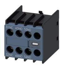
Auxiliary switch on the front, 2 NO + 1 NC Current path 1 NC, 1 NO, 1 NO for 3RH and 3RT screw terminal 31/32, 43/44, 53/54 Special inscription
