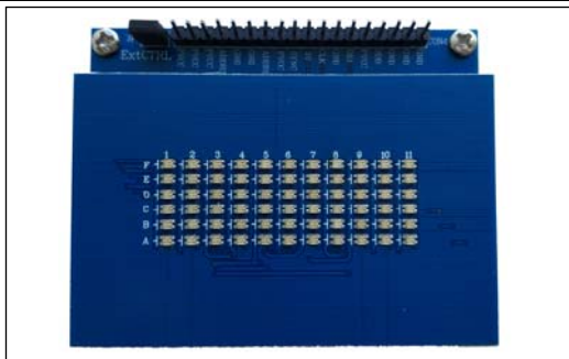
Figure 1: Photo of IS31FL3743A Evaluation Board
