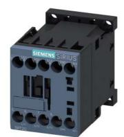
Power contactor, AC-3 9 A, 4 kW / 400 V 1 NC, 12 V DC 3-pole, Size S00 screw terminal
