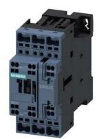
Traction contactor, AC-3 12 A, 5.5 kW / 400 V 1 NO + 1 NC with electronic drive 72 V DC, 0.7-1.25\* US with integrated varistor 3-pole, Size S0 Spring-type terminal
