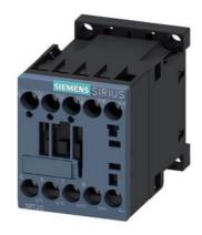
Power contactor, AC-3 7 A, 3 kW / 400 V 1 NC, 24 V DC communication-capable, 3-pole, Size S00, screw terminal
