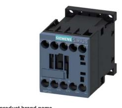
power contactor, AC-3 7 A, 3 kW / 400 V 1 NC, 24 V DC 0.7-1.25\* US, 3-pole size S00, screw terminal suitable for PLC outputs not expandable with auxiliary switch
