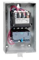
Non-reversing motor starter, Size 1 3/4, Three phase full voltage, Solid-state overload relay, OLR amp range 10-40A, 110V 50Hz / 120V 60Hz coil, Non-combination type, Enclosure type 1, Indoor general purpose use, Standard width enclosure
