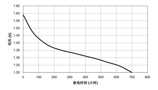
Discharge method: 33k $\Omega$ , 24hours/day, E.V. 1.2V Temperature: 20±2 $^{\circ}$ C
