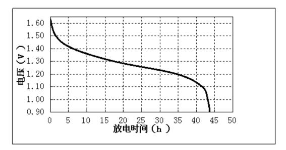
Discharge method: 6.5k $\Omega$ , 24hours/day, E.V. 0.9V Temperature: 20±2 $^{\circ}$ C
