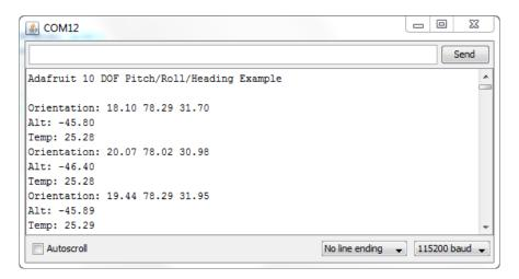
This raw data shows the main orientation data, consisting of 'roll', 'pitch' and 'heading' (or 'yaw) in degrees, followed by the current altitude and temperature if you are are using the 10-DOF breakout (the 9-DOF and LSM9DSO breakouts can't measure
