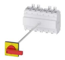
SENTRON, Switch disconnector 3LD, emergency switching-off switch, 6-pole, lu=250 A, operating power / at AC-23 A 400 V: 132 kW, floor mounting with door coupling, knob-operated mechanism, red/yellow, 4-hole mounting of the handle
