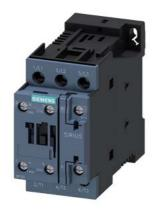
power contactor, AC-3 12 A, 5.5 kW / 400 V 1 NO + 1 NC, AC (50-60 Hz) DC operation 21-28 V AC/DC, 3-pole Size S0, screw terminal
