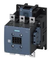
Contactor, AC-1, 400 A/690 V/40  $^\circ\text{C},$  S10, 3-pole, 200-220 V AC/DC, with varistor, 2 NO+2 NC, Connection rail/ screw terminal
