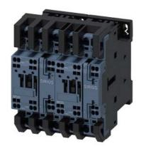
Reversing contactor assembly AC-3,5,5 kW/400 V,AC24V,50/60Hz 3-pole, Size S0 Spring-type terminal electrical and mechanical interlock
