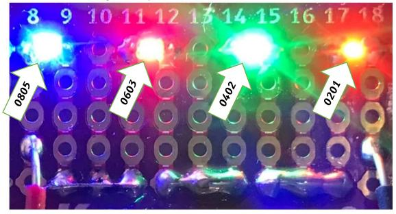
The LEDs were powered in series at 10mA
