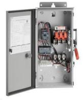
Slim Line Pump Control Panel NEMA size 1 Three phase full voltage Solid-state overload relay OLR amp range 3-12A 220/230V 50/60Hz Coil 30A fusible disconnect 30A/250V fuse clip 1NC / 1NO auxiliary contacts HOA Sel. Sw. <(>&<)> Start/Stop 3-point power terminal block 3-point control terminal block 3-point ground lug Enclosure NEMA type 3/3R Weather proof outdoor use
