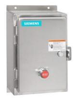
Non-reversing motor starter Size 0 Three phase full voltage Solid-state overload relay OLRelay amp range 3-12A 240VAC 50HZ / 277VAC 60HZ coil Combination type Water/dust tight non-corrosive
