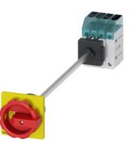
Load disconnector 3LD3, lu 63 A Main switch 3-pole + N Rated operating capacity at AC-23 A at 400V 22.0 kW floor mounting Basic switch with door coupling Central hole mounting 22.5mm Rotary actuator red / yellow 66 x 66 mm
