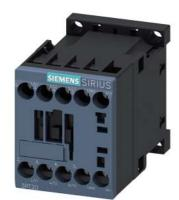
power contactor, AC-3 9 A, 4 kW / 400 V 1 NO, 24 V DC 0.7-1.25\* US, 3-pole, size S00, screw terminal suitable for PLC outputs not expandable with auxiliary switch
