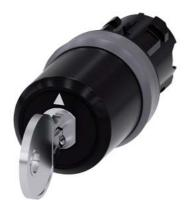
key-operated switch Siemens, 22 mm, round, plastic with metal front ring, lock number SSG10, with 2 keys, 3 switch positions I>O<II, momentary contact on the left, latching on the right, actuating angle 2x45°, 10:30h/12h/13:30h, key removal II
